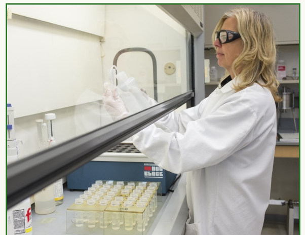
Lynn Aldridge, State Hygienic Laboratory environmental lab analyst, prepares samples so they may be used to test for levels of arsenic in drinking water.
